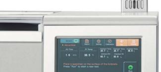
The DryRate 201 testing conditions are constantly monitored by the built-in anemometer (air flow sensor) and infrared thermocouple probe.
